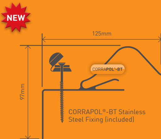
CORRAPOL-BT Foam Eaves filler: 930 x 25 x 40mm
