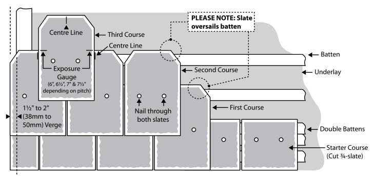
Verge slates should oversail the brickwork/barge board by 11/2" (38mm), and may need to be cut to size at either end.
