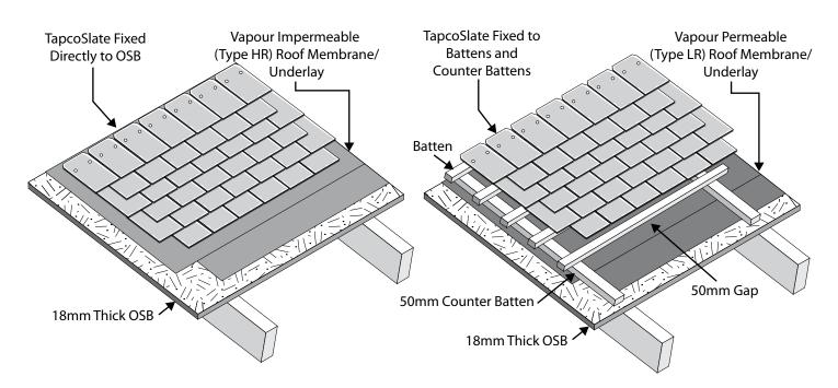
Being a laminar product, TapcoSlate repels water and does not absorb it, this means that water penetration is non-existent from the roof surface itself. However, vapour/air barriers minimise the risk of moisture accumulating on the underside of the slates/OSB as the most common source of moisture is generated inside the property itself. Using a **vapour impermeable** roof membrane/ underlay reduces this risk even further.
