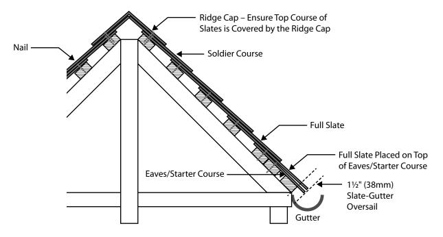
The required gauge and number of courses can then be calculated. The first course should sit on top of an eaves course. Double batten as shown in the diagram to accommodate the eaves slates.
