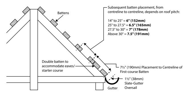
The distance from the first course batten to the second course batten, and beyond, is dependent on the roof pitch and subsequent slate exposure gauge settings. Please see the diagram of the TapcoSlate and the Pitch, Gauge, and Coverage table on page 4. The diagram above also shows an approximate guide to subsequent batten placement.
